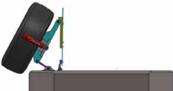
Figure 4. The spare wheel carrying mechanism when the back door is opened
