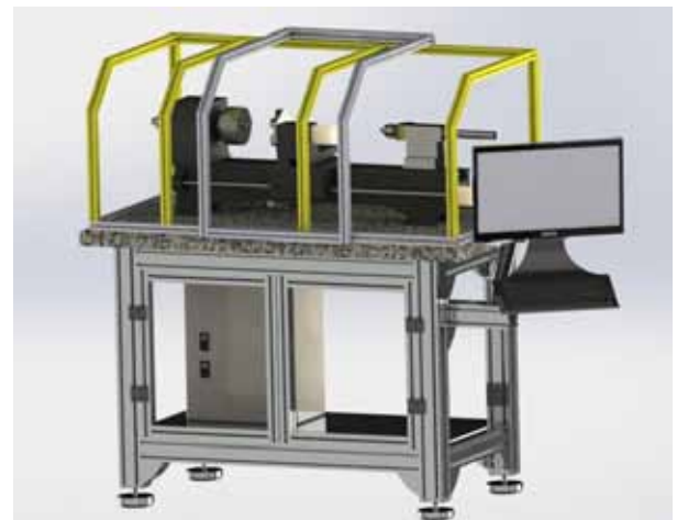
Figure 2: Assembled components of the CNC lathe with enclosure.
