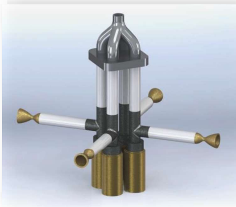
Figure 2: Poppet Valve Design [2]
