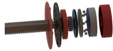
Figure 3: The brake fitted on the threaded cylindrical shaft along with the encoder.
