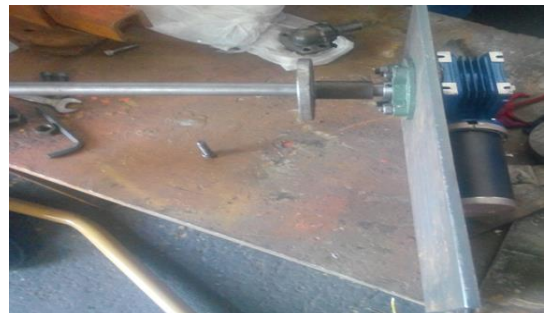
Figure 7: Assembly process of Motor-Gearbox-Bearing-Shaft-Weld Neck Flange on the side support
