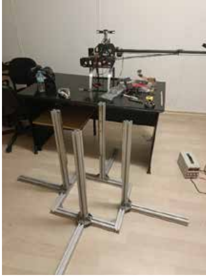
Figure 5: Rigid Base Structure with Elevational Mechanism
