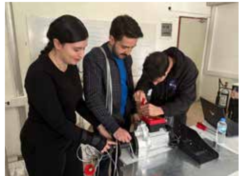
Figure 19: Motor preparation process through partial disassembly of components before installation.
