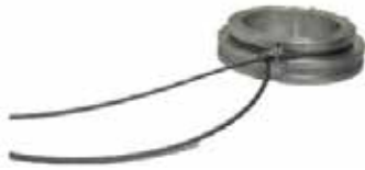
Figure 14: Connection of rope 1 to lower flange 2
