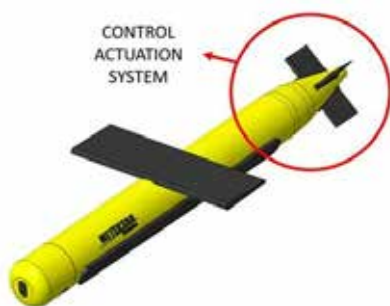
Figure 1: General Structure of the Underwater Towed Body
