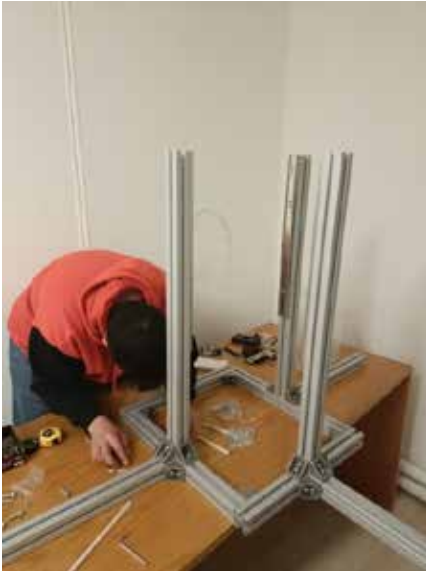
Figure 6: Assembly process of base structure with corner bends and allen bolts
