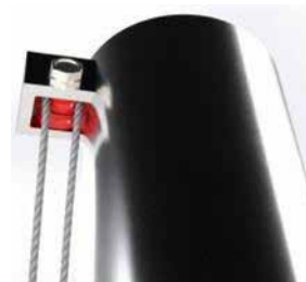
Figure 13: Mounting of pulley 1 into pulley housing
