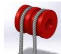
Figure 12: Rope 1 winding around pulley 1
