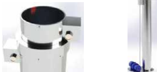
Figure 17: Mounting of upper flange 1 onto tube 1 and fixing rope 1 to the motor line
