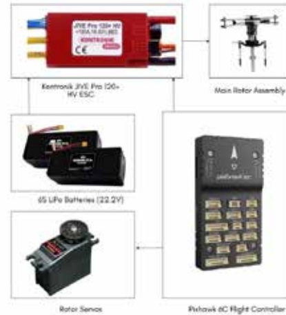
Figure 4: Power and signal architecture.
